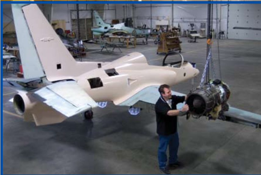
Rob Huntington is getting ready to install a GE engine in a Viperjet kit plane.
