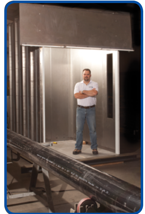
Richard Vice is standing in an elevator cab with a hydraulic shaft in the foreground.
